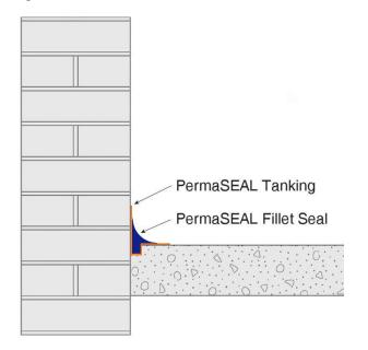
Cut a chase into the floor at the wall floor joint 20mm x 20mm deep cutting into the wall where possible. Then follow the preparation guidelines, once clean apply a coat of PermaSEAL Tanking to the area 100mm up the wall across the chase and 100mm onto the floor. Whilst still tacky apply PermaSEAL Fillet Seal to the area and chase, rounding off the fillet to create a smooth curve across the junction. Allow to dry for at least 1 hours before over coating.
